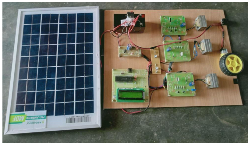
Figure 3: Hardware Implementation to charge Electric vehicle from Solar Panel
